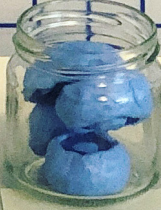
SILICON RINGS MADE BY CASTING COW'S MILK BEADS FOR A TEXTURE
