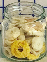
CASEIN PLASTIC BEADS MADE FROM FRESH COW'S MILK WITH VANILLA, AND DYED WITH SPICES
