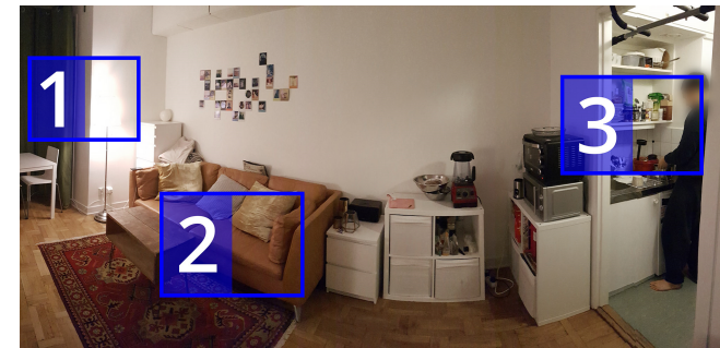
Figure 1: Diagram of sensor locations in our studio apartment. A photocell (remains) is within the floor lamp (1), a soft potentiometer (removed) was tried in various couch locations (2), and a temperature sensor (removed) was above the stove (3).
